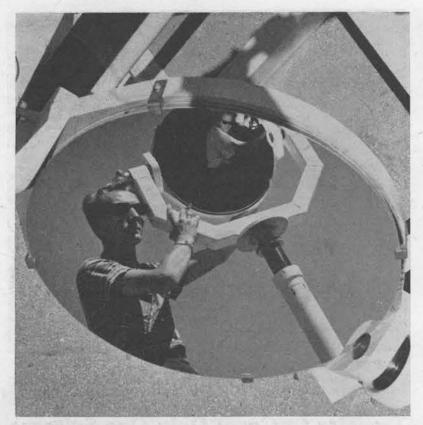
MIRROR SYSTEM shown in the photograph above reflects a constant beam of light through a tube in the wall of Bldg, 880 into the optical development laboratory of 7224-1. Large mirror rests on the ground and tracks the sun. Second mirror, being positioned by Bob Hughes, beams the light through the tube where Dan Fenstermacher is checking alignment with the optical bench inside.
